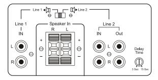
There are a total of 4RCA inputs on the back panel of the MI5 Powered Amplifier. These RCA inputs are labeled as "Line 1 Input" and "Line 2 Input". They are also designated with an "R" or an "L" as Right channel or Left Channel inputs respectively.
