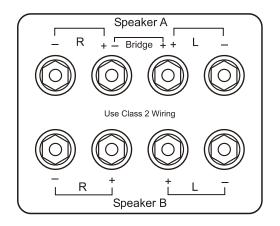
NOTE: Only one pair of channel s can be bridged together. Do not attempt to bridge both A&B speaker terminals, as this may result in a lower impedance than the amplifier is designed to accommodate, and may damage your amplifier. The minimum impedance for the total load connected to a pair of channel s in the bridged mode is 8-ohm.
