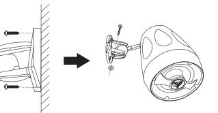
When mounting the speaker to the wall, make sure the proper screws / bolts
