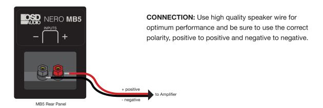
**NOTE:** The wire for both speakers should be about the same length. If one speaker is placed closer to the amplifier than the other, hide the excess wire behind the amp.
