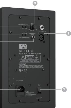
1 JACK TRS, XLR INPUT (BAL/UNBAL). The system accepts JACK TRS or XLR input connectors. These balanced inputs can be used to connect balanced or unbalanced audio sources at line level.
