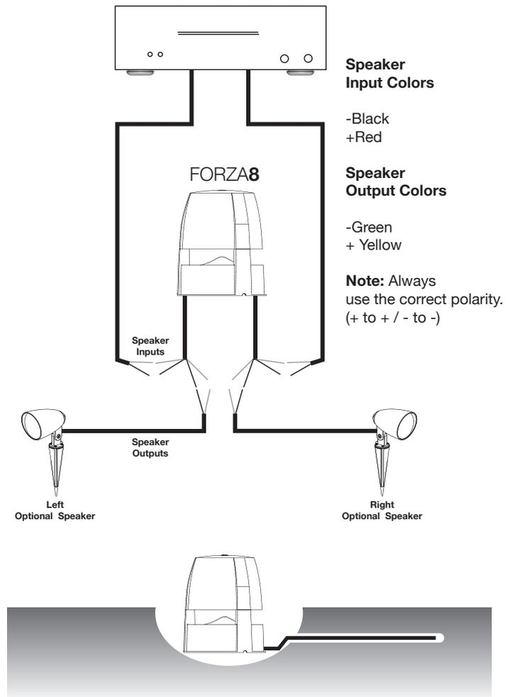
To complete installation, place the subwoofer in a pre-dug hole and run the speaker leads to the speakers and amplifier by trenching wherever necessary to hide/protect the wires. Fill the hole after testing the newly installed system.
