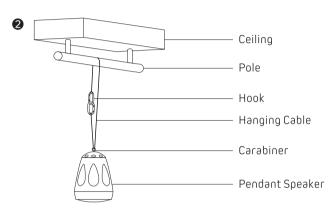
Make sure the speaker is properly secured to the ceiling /  $\angle$ !\tag{\text{building}} building's structure. please use the proper screws, bolts, or anchors (not included). Failure to do so may cause the speaker to become unsecured &cause potential damages/ injuries.
